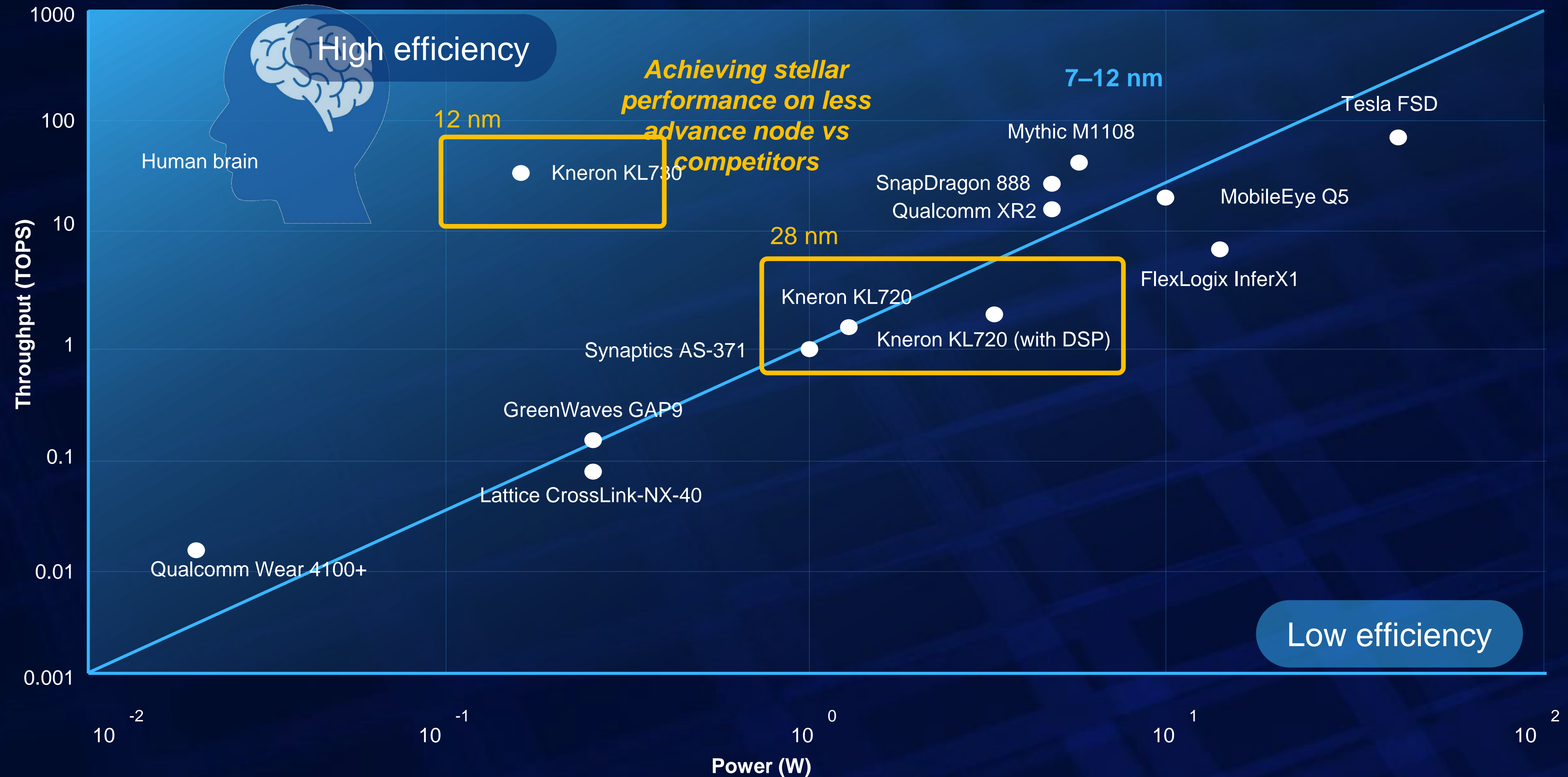
Figure 9: Throughput comparison of different commercial edge processors for NN inference at the edge.
